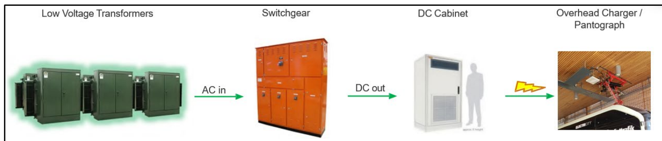
Figure 1: Battery-Electric Charging Infrastructure Overview 5
