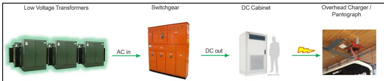
Figure 1: Battery-Electric Charging Infrastructure Overview 6
