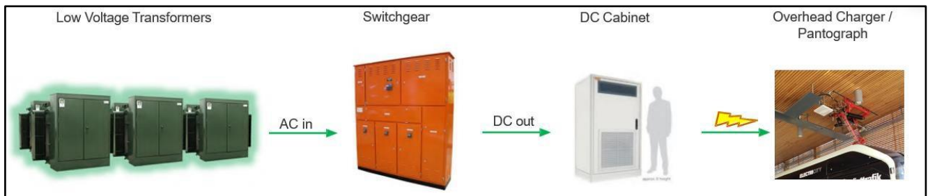
Figure 1: Battery-Electric Charging Infrastructure Overview
